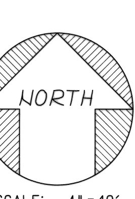
BEARINGS SHOWN HEREON ARE BASED ON TRUE BEARINGS (FLORIDA STATE PLANE COORDINATES SYSTEM - EAST ZONE - NAD 27) AS SHOWN ON THE PLAT OF THE COASTAL CONSTRUCTION CONTROL LINE, PLAT BOOK 9, PAGE 99, RECORDED JULY 9, 1985; LYING BETWEEN DEPARTMENT OF NATURAL RESOURCES RANGE MONUMENTS "R-9G" AND "R-97".
